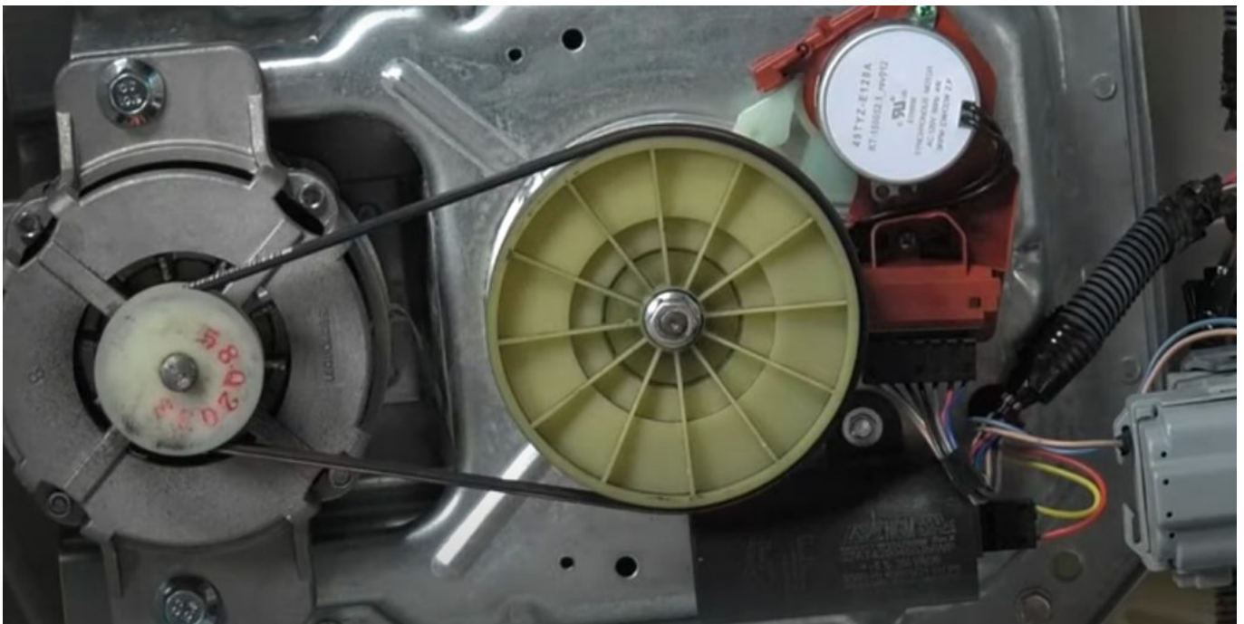
Check and Adjust the Drive Belt
